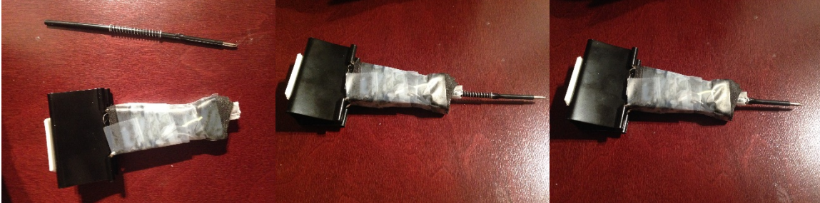
Figure A: Shows the writing utensil mechanical design the large case is a weight used to keep the pen touching the ground. The spring in the pen is used to keep the vibrations away from the writing as the robot is riding across the canvas. This system allows for an easy replacement of the pen if the ink was to run out.
